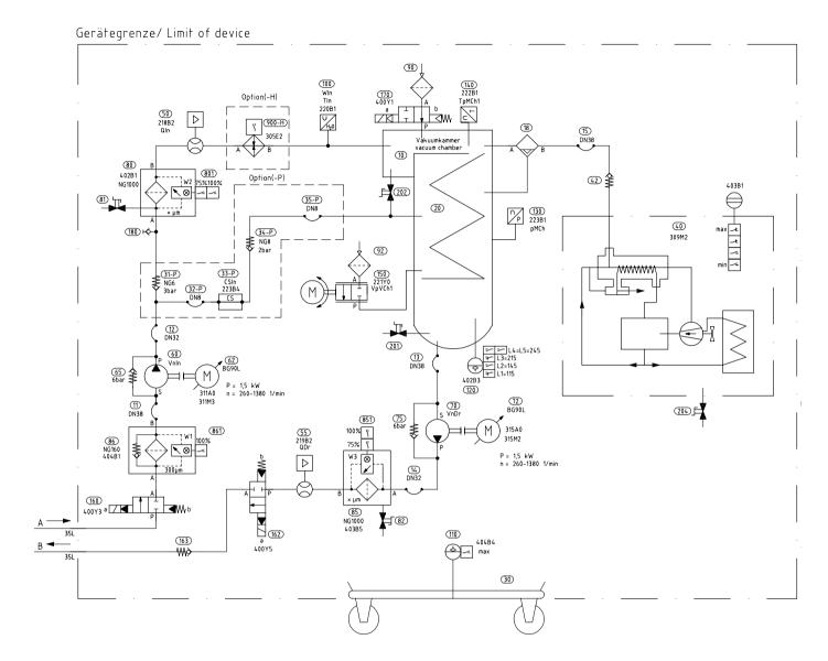
The ABVCM system removes dirt, oil aging products, gases as well as free and dissolved water from hydraulic andlubricating oils in a multi-stage process.
